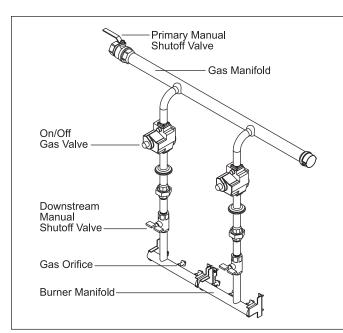
Figure 5. Typical Gas Train Configuration.
